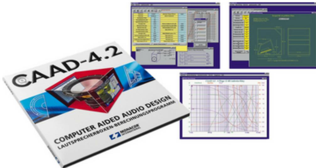
This simulation software offers more than just the basic presentation of acoustic results to be expected. An essential part of the function is that recommended cabinet dimensions are optimised. These cabinet forms meet the complex requirements concerning speaker dimensions, volume and bass-reflex openings which may exist regarding diameter and length. These cabinet forms also correspond to a favourable distribution as far as possible of cavity resonances and to a reduction of air flow noise.
